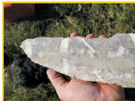
White laths of spodumene with feldspar, quartz and muscovite. International property, Bouvier showing. UTM Coord.: Easting: 714525; Northing: 5370634; NAD83; Zone 17N.
