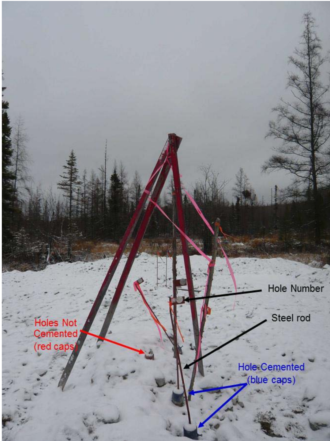
FIGURE 10-1 IDENTIFICATION OF HOLE COLLARS AND CASING CAPS
