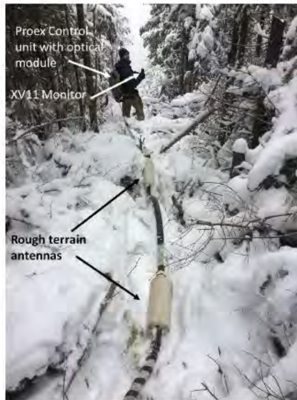
Figure 2: Rough terrain antennas attached to the operator which transports the ProEx Control unit and its optical module inside a backpack and carries the XV11 Monitor in front.
