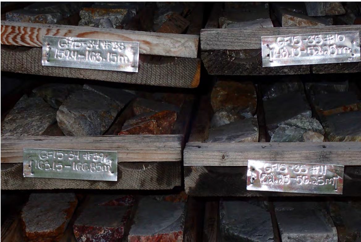
Photo 12: Core Boxes at Core shed with Identification
