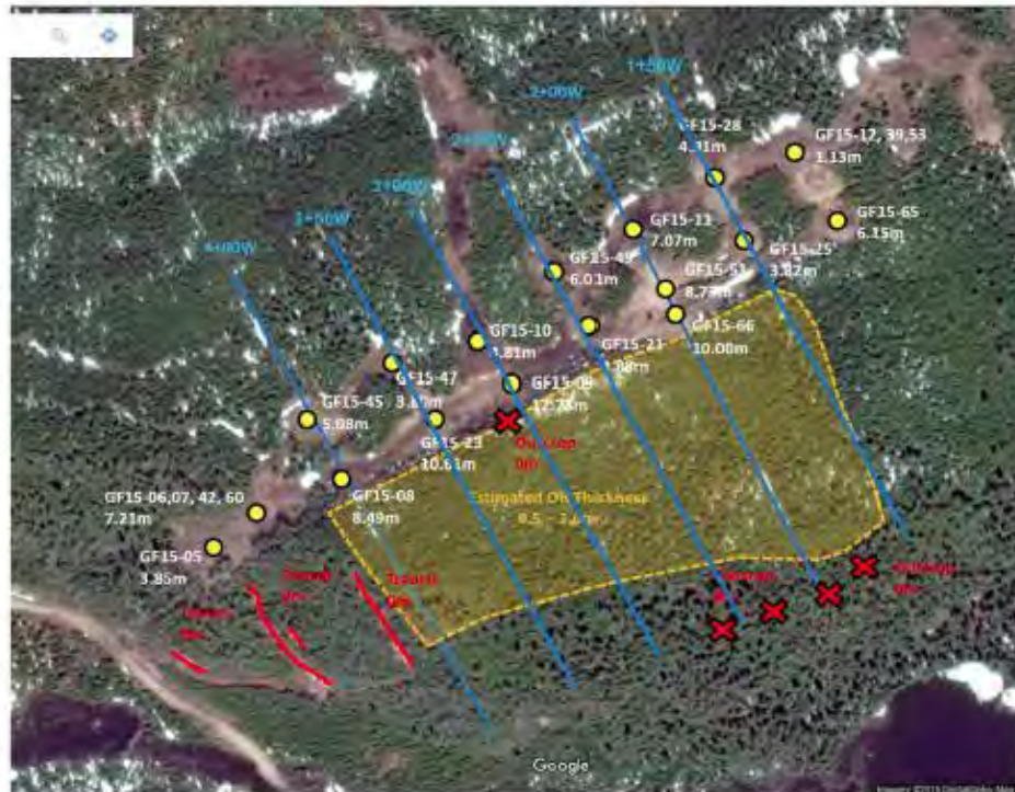
Figure 3: Location of the grid lines and available prior information on overburden thickness in the survey area
