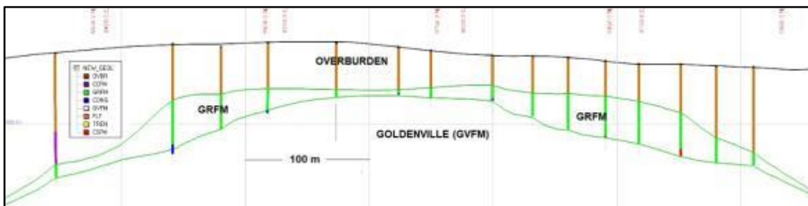
Figure 14-4: Section View – Getty, Looking SE
