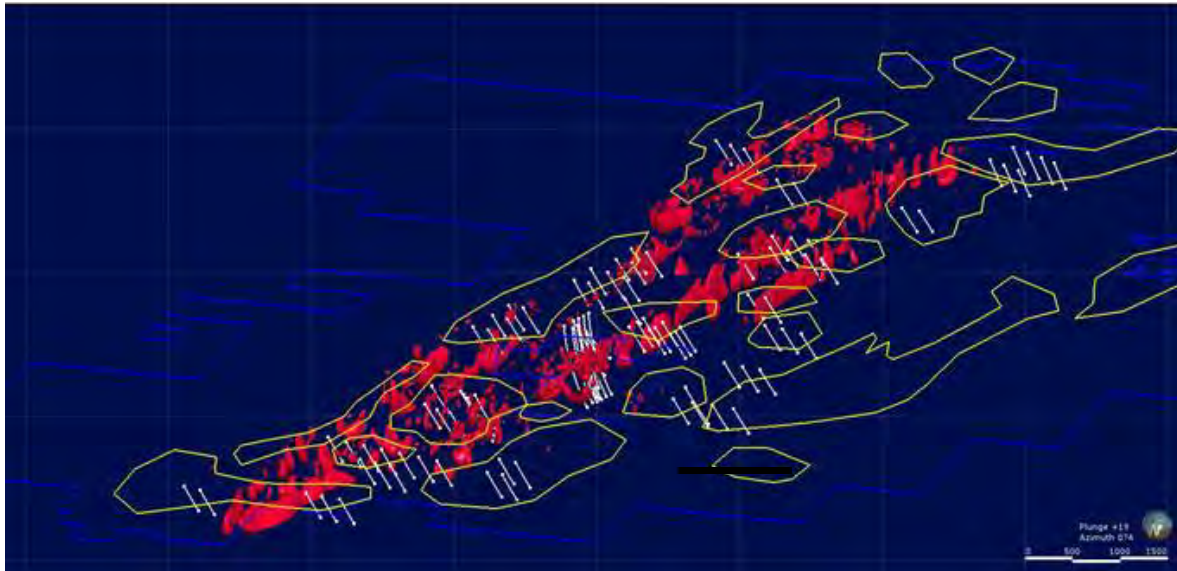
Figure 3. 3D IP survey showing chargeability iso-surfaces (red) across entire survey area with planned Phase 1 and 2 drill holes and 2017 MMI Soil Geochemistry Anomalies (yellow)
