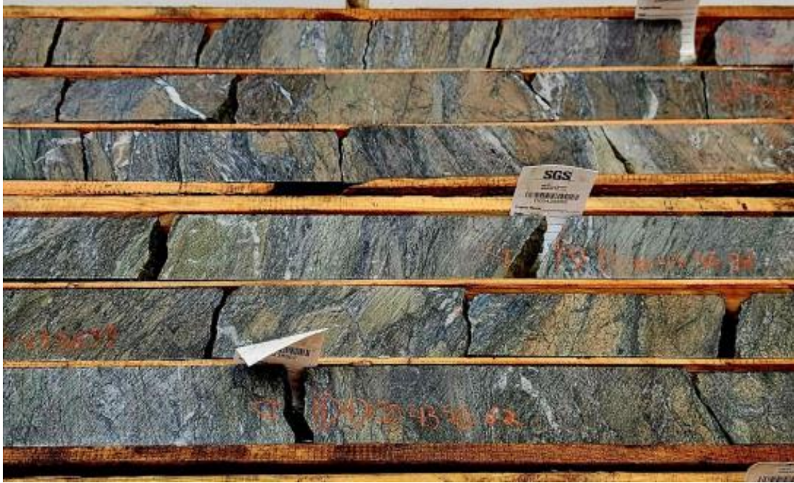
Image 2: Replacement Style Mineralization, DQ23-02 recovery was 90% from 10.65 m of 4.0 g/t Au (Includes 5.0 m of 5.3 g/t Au)
