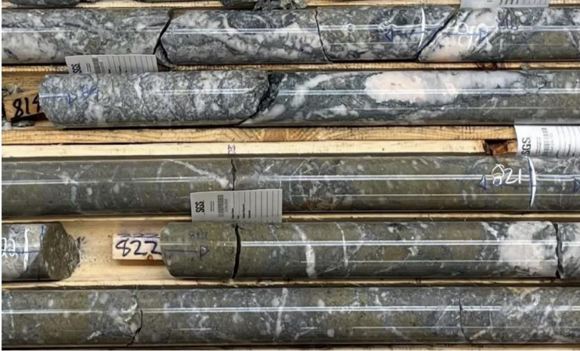
Image 4: Quartz-Feldspar Porphyry Related Mineralization, DQ23-02 recovery was 76% from 25.0 m of 1.7 g/t Au.
