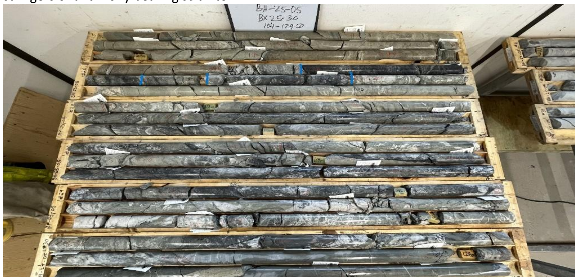
Photo 1: Mineralized Section in Drill Hole BH-25-05. Note stibnite is identified over 20 meters in this hole.
