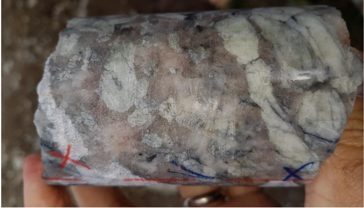
Figure 7-4: Drill core from hole AL-16-10, showing spodumene mineralization in the new Authier North pegmatite
