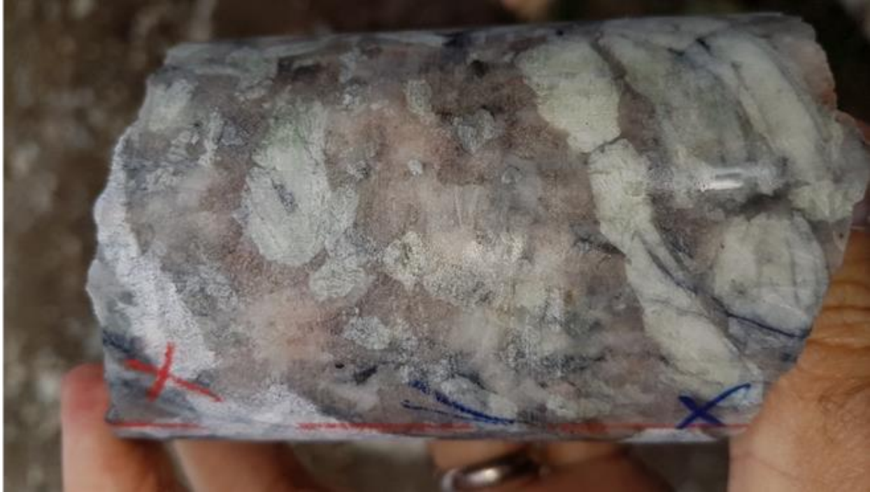
Figure 10-7: Hole AL-17-10 in the Northern Pegmatite which intersected 7 m of 1.36% Li 2 O from a downhole depth of 15 m (vertical depth of 12 m), including 2 m of 2.24% Li 2 O from 17 m
